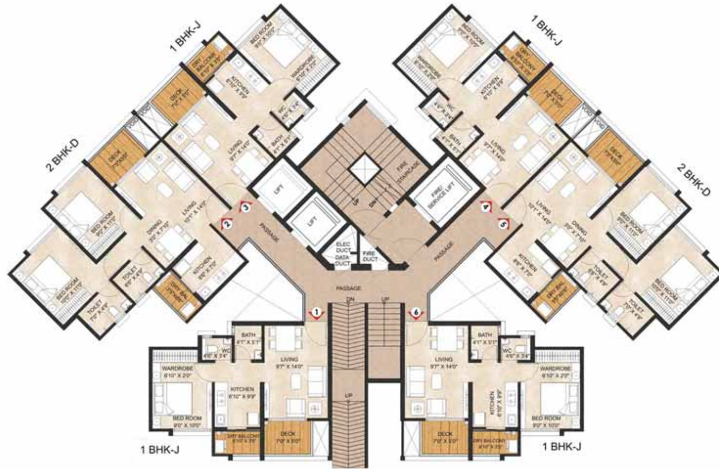
TP1 FIRST FLOOR PLAN BUILDING NO 18
